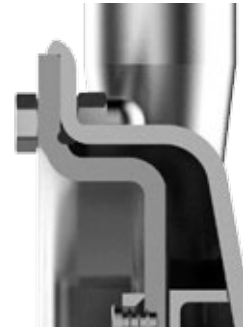
O-ring sealing between pump housing and cover
