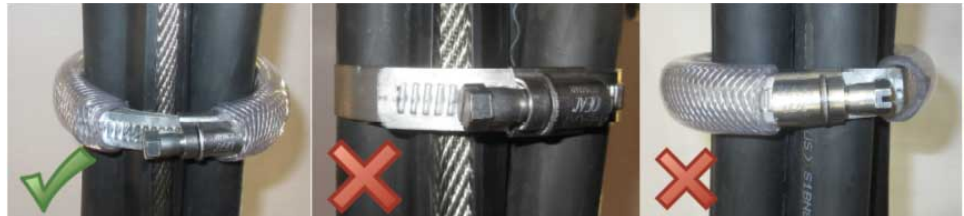
Fig. 18: Installation information for the cable clamps
