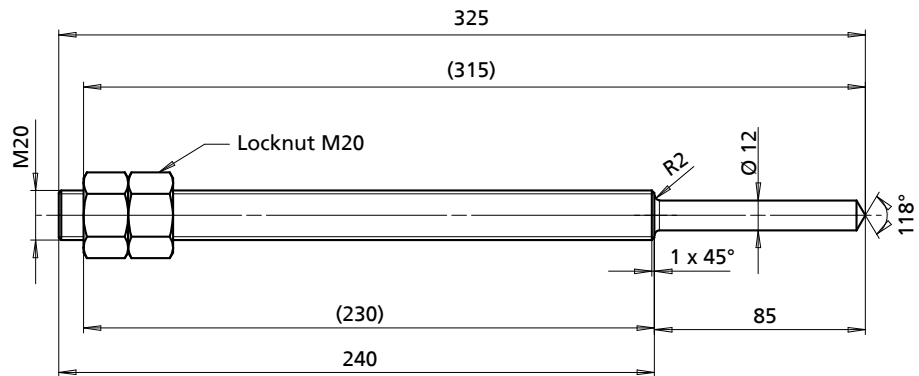
Fig. 30: Forcing screw M20 x 325
