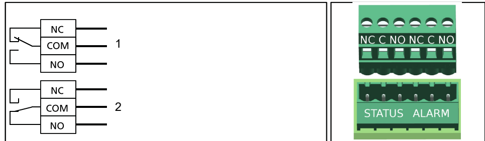
Fig. 11: Wiring diagram for the general fault message
