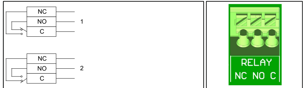
Fig. 16: Wiring diagram for the general fault message
