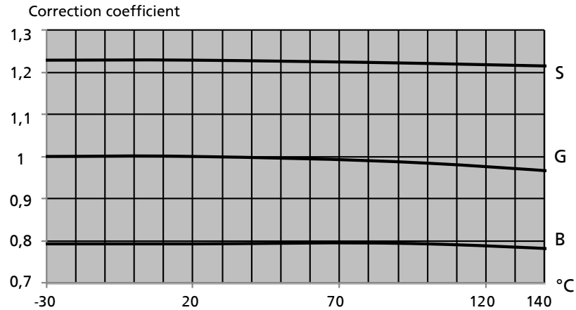
Fig. 11: Temperature/material correction diagram for casing materials G (EN-GJL-250/A48CL35B), S (EN-GJS-400-15/A536 GR 60-40-18) and B (CC480K-GS/B30 C90700)
