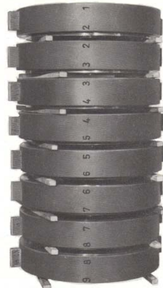
Figure 30 – Stacking the stage casings
